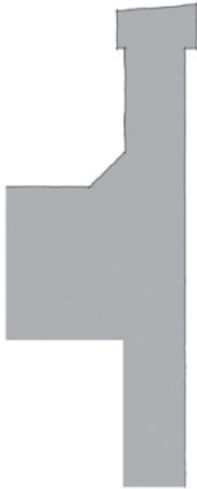
Simple parapet with Stone or Brick Cap
