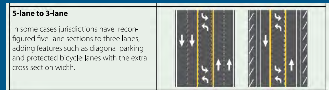
Figure 2. Typical Road Diet Basic Design
